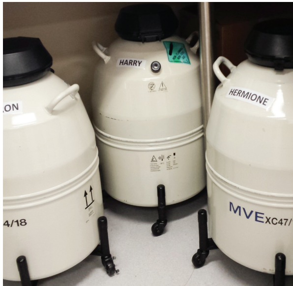
Figure 1: Tanks in the laboratory that contain frozen embryos and sperm stored at -196^{\circ}\text{C}
